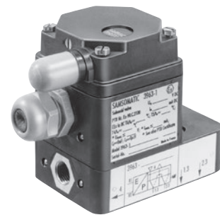
Fig. 1: 5/2-way solenoid valve · Actuated on one side · With spring return mechanism · K_{VS} 0.16 · G \frac{1}{4} connection
